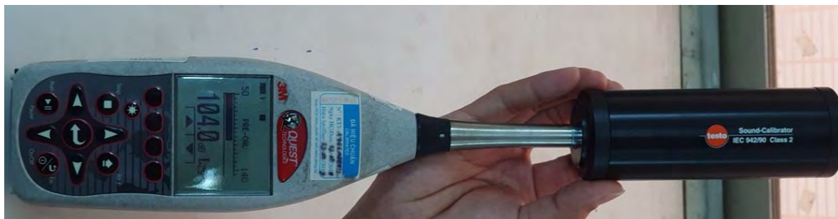
Figure 13. Noise meter instrument & calibrator
