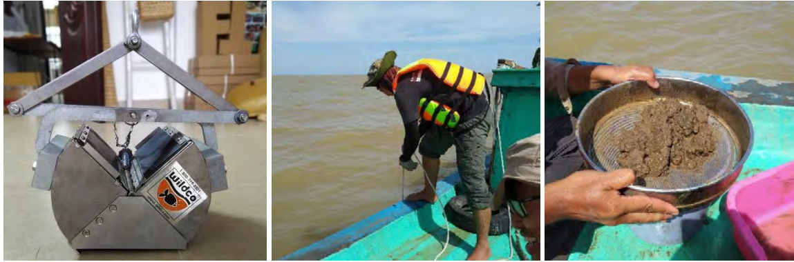
Figure 13: Ponar grab (footprint 15cm x 15 cm) used for macrobenthic sampling
