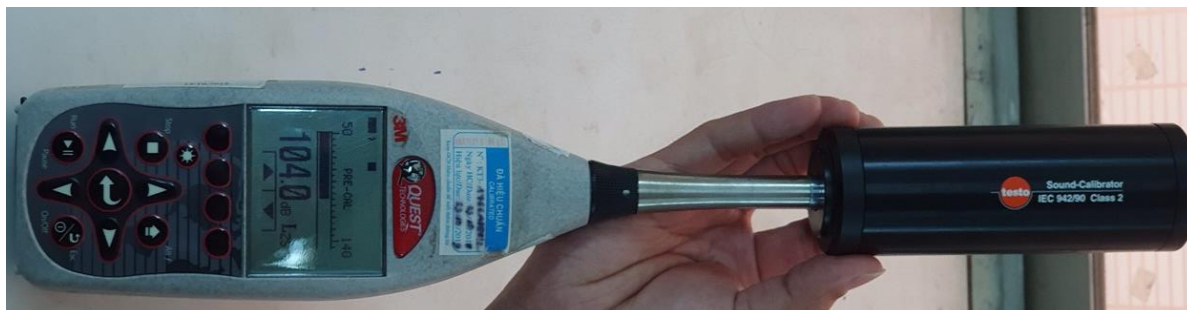
Figure 13. Noise meter instrument & calibrator
