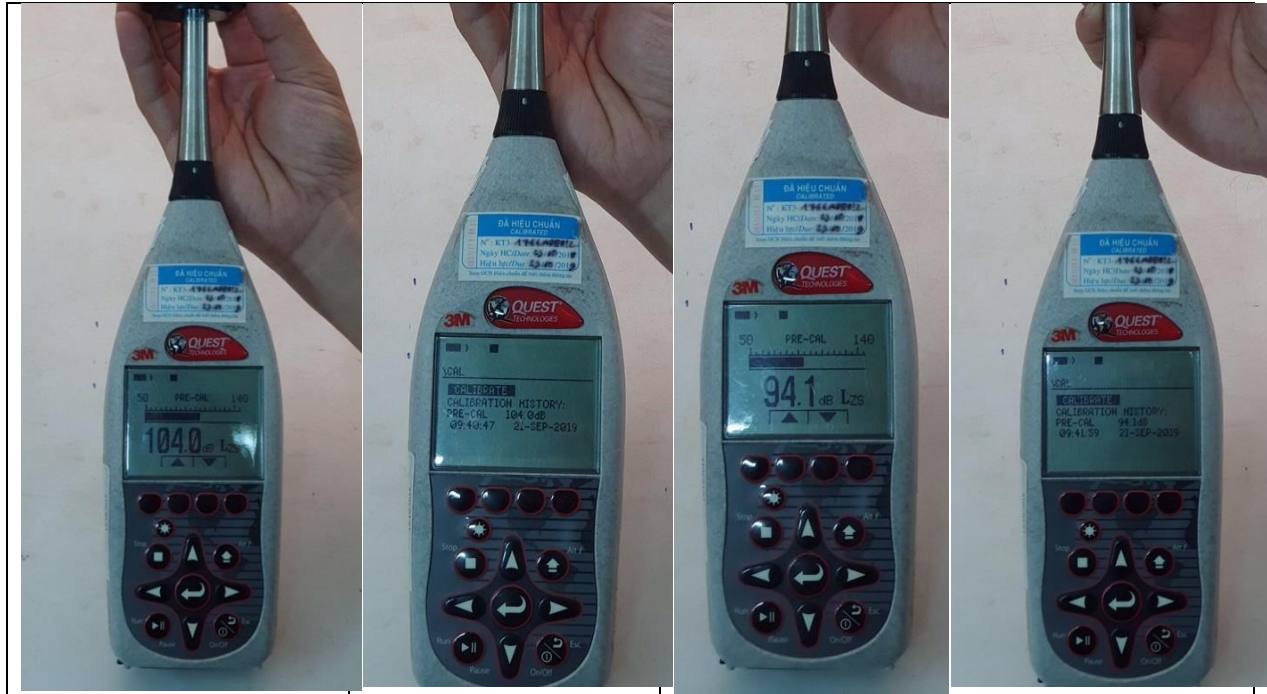
FIGURE C1. CALIBRATION IN THE LAB
