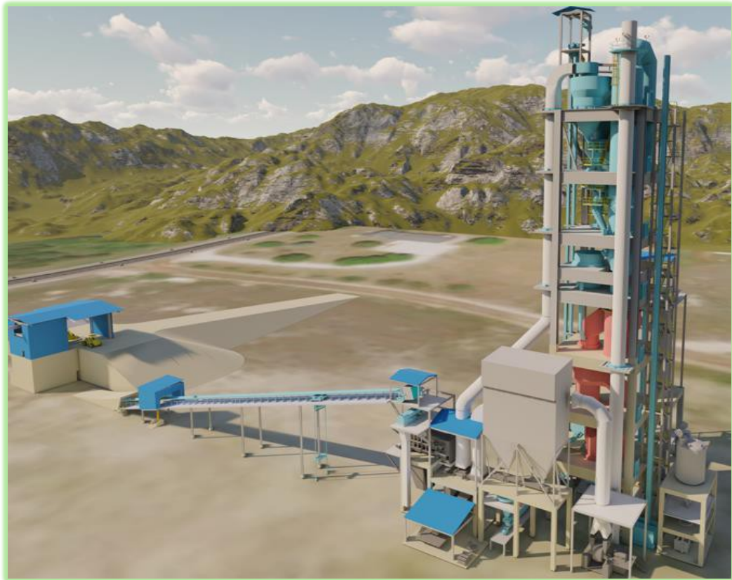
Figure 3-14: 3-D View of clay calcination installation
